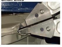
Take small bites, close the tool and move it deeper into the seam.
