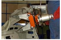
Close the tool, move it along the joint and re-engage
