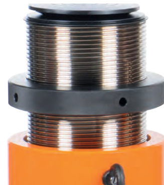
Multiple-start and rounded thread on plunger for a quicker positioning of the locknut and easy dirt removal
